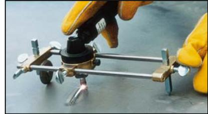
The Deluxe torch guide kit for circles of 45 to 1050 mm diameter. Centre is fixed by pin, magnet or suction cup. Also for straight line cutting.
